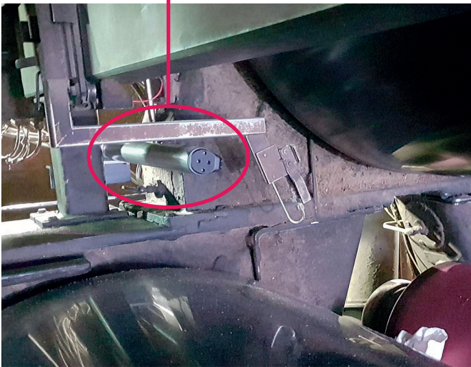
Extended detection distance decreases risk of mechanical sensor damage.
