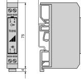
Fig. 9. SINEAX TI 816 on G-type rail EN 50 035 – G 32.
