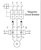
Overload protection of the motor is easily achieved by installing a manual thermal magnetic circuit breaker on the supply side of the motor.
