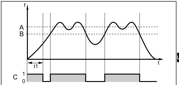
A = requested flow; B = switch point; C = output relay t1 = power-on delay time
