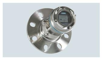
SITRANS LR560 2-wire, 78 GHz FMCW radar level transmitter for continuous monitoring of solids and liquids to a range of 100 m (328 ft).
