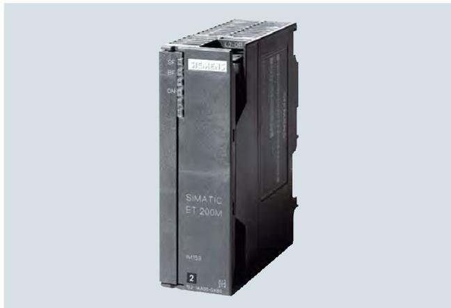
The ET 200M system with various interface modules is available for the distributed use of S7-300 I/O modules. Depending on the application purpose, the best suited IM in terms of costs and functions can be selected:
