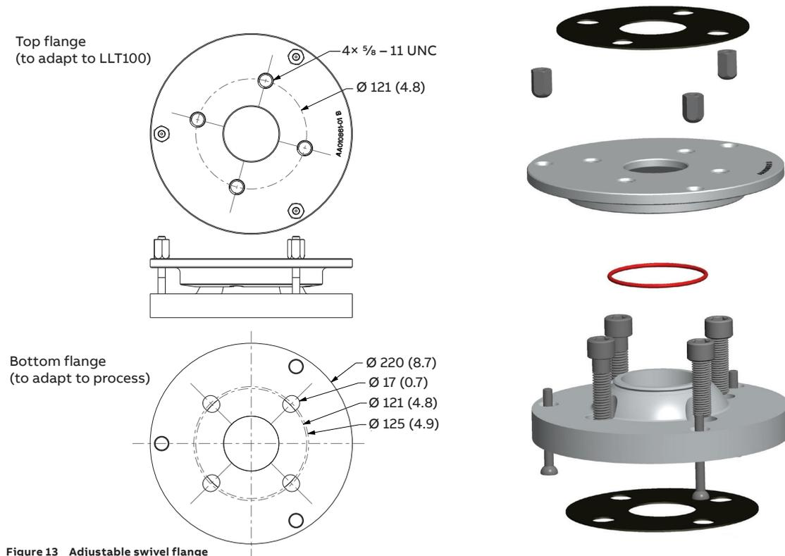
Figure 13 Adjustable swivel flange
