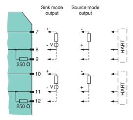
Short circuit unused circuits on the output. Open circuit outputs increase the internal power dissipation by up to 300 mW per channel.
