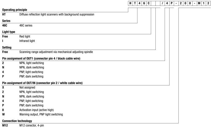
200-M12 Cable 200 mm with M12 connector, 4-pin
